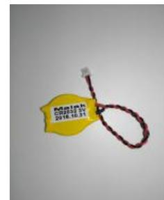
Figure 2.2-9 RTC battery
