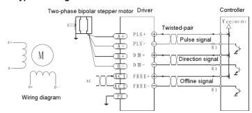
Note: when above V1.4 version, R1=0, no need to weir 2Kohm resistor.
